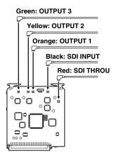
7 Insert the SDI board in the F3 slot located on the rear panel side.
