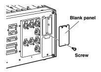
5 Attach the accessory connector board to the rear panel. As shown in the diagram below, after passing the connecting cables through the hole provided for the F3 slot, plug them into the top section of the connector board and then fix the connector board in place using the screw.
