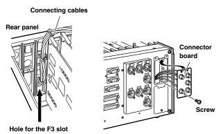
6 Connect the connecting cables to the SDI board.
